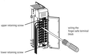
When wiring the terminal block, keep the finger-safe cover in place.
