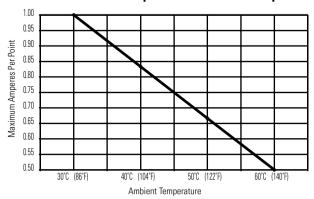
1769-0B16 Maximum Amperes Per Module vs. Temperature
