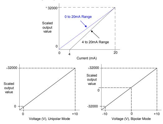
The resolution per bit depends on the channel's configured range:
