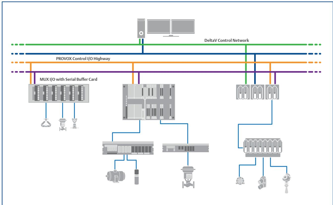
The S-Series DeltaV Controller Interface for PROVOX I/O.
