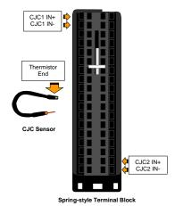
The thermistor end of the CJC sensor must be installed in the CJC1 IN+ or CJC2 IN+ terminal for accurate temperature measurements. The gold pin end of the CJC sensor must be installed in the CJC1 IN- or the CJC2 IN- terminal.
