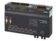
\*\*\*\*\*\*\*\*\*\* spare part \*\*\*\*\*\*\*\*\*\* OSM TP62 Optical Switch Module with two FOC ports 100 Mbit/s, 6 RJ45 Ports 10/100 Mbit/s and eight digital inputs, redundant 24 V DC infeed, signaling contact integrated redundancy manager with network management
