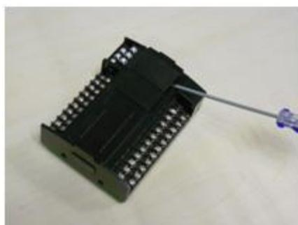
**Figure 4-3 the Removal of Cover**
