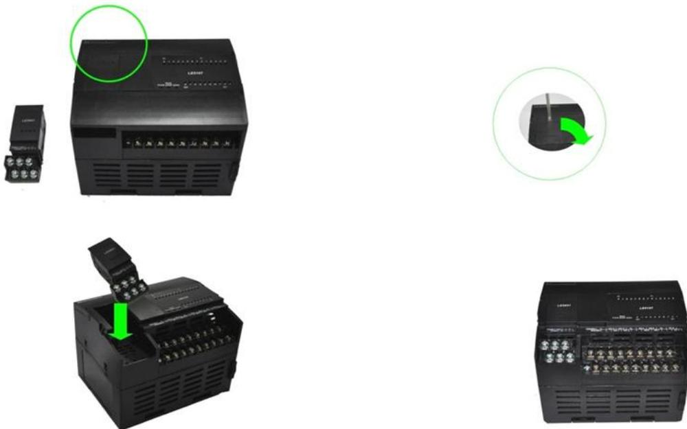
**Figure 12-11** *Installing an Expansion Board*
