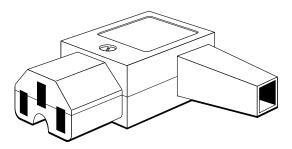
Figure 2-1. AC Power Connector.
