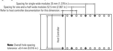
Locate holes every 17.5 mm (0.689 in.) to allow for a mix of single-wide and one-and-a-half-wide modules (e.g. 1769-OA16).
