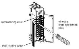
When wiring the terminal block, keep the finger-safe cover in place.
