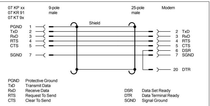
Fig. 10.2-4: Terminal assignment 07 SK 92
