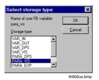
Every user function block variable has a storage type. The storage type determines how the variable is used inside the user function block. The storage type determines where the runtime value of the variable is to be found.
