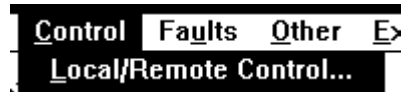
Figure 10 - 1. Pull-down menu for Control. Note that the menu command may be inactive if it is not possible to use it in the current situation.
