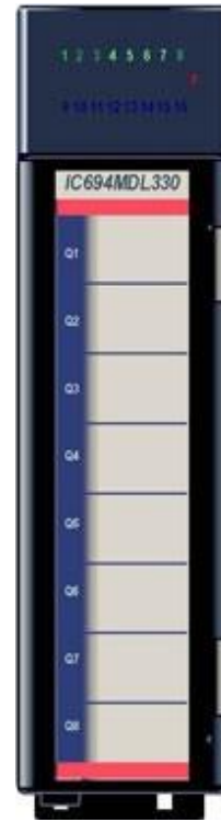
Figure 35: 120/240 Vac 2A 8-Point Isolated IC694MDL330
